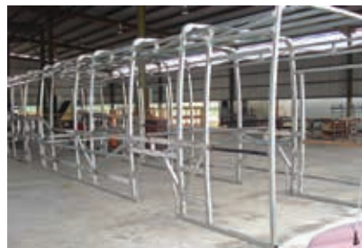
◀ Bus structure build to ADR 59 standard
