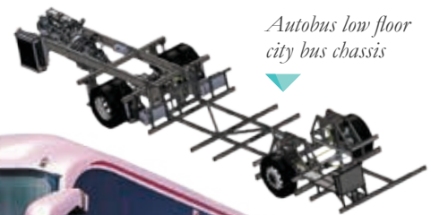
◀ Bus structure build to ADR 59 standard
